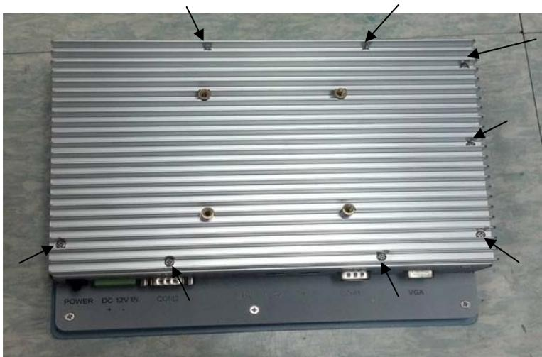
Step 2: Loose the three specified M3 screws to get the Hard Disk Drive (HDD) bracket.
