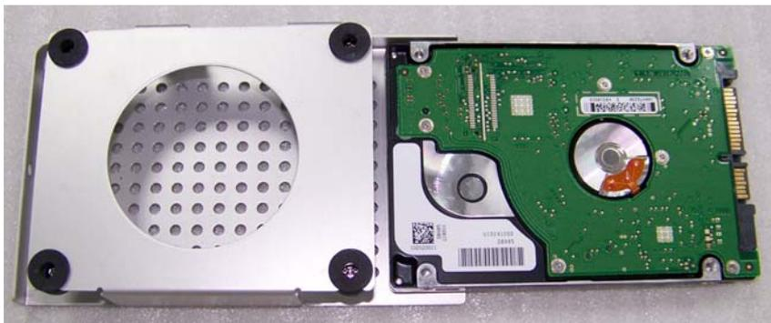
Step 4: Fasten the four screws to fasten the HDD and the HDD bracket
